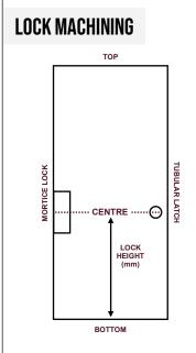
\*The Lock Height (mm) for both a Mortice Lock and a Tubular Latch is the measurement from the bottom of the door to the centre of the lock cut-out.
